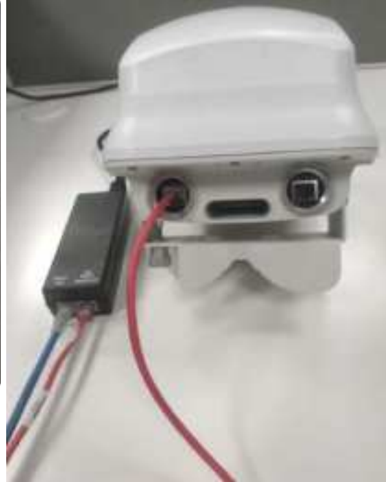
Figure 135: Connecting the V2000 power injector
