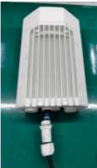
Figure 122: Connecting the input side of AC/DC PSU
