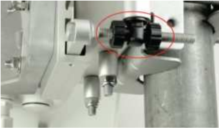
Figure 96: Moving the azimuth adjuster
