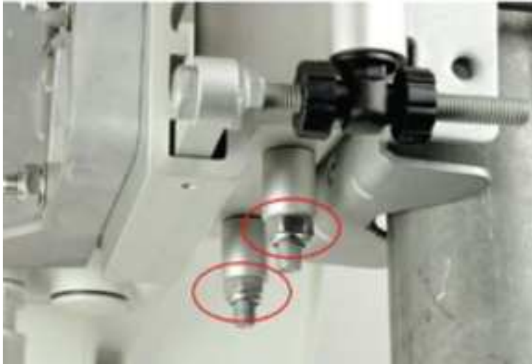
Figure 94: Two Nyloc screws in the azimuth
