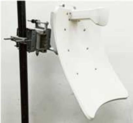
Figure 92: Locking the antenna alignment
