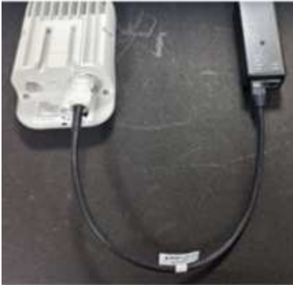
Figure 134: Connecting the V1000 Power injector
