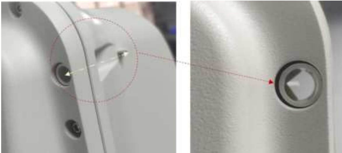
Figure 78: Aligning the V2000 device
