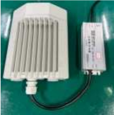
Figure 123: Connecting the output side of AC/DC PSU
