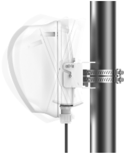
Figure 80: Using the adjustable bracket knob for alignment
