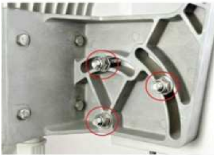
Figure 93: Three Nyloc screws on the unit
