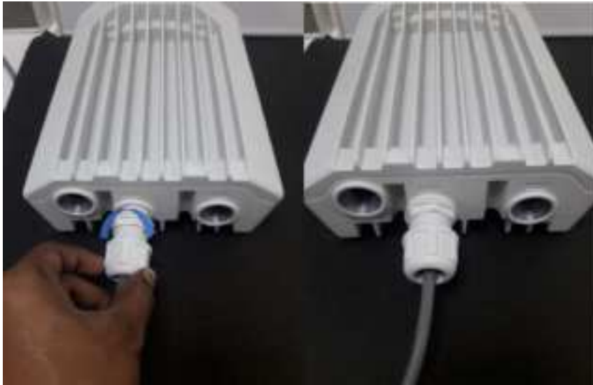
Figure 114: Rotating the gland
