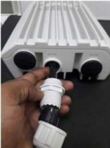
Figure 117: Removing the latch of the RJ45 plug
