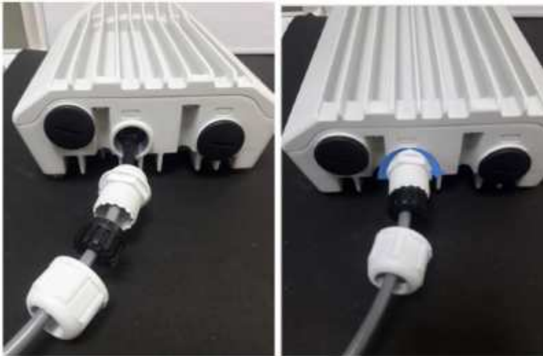
Figure 113: Connecting the RJ45 plug
