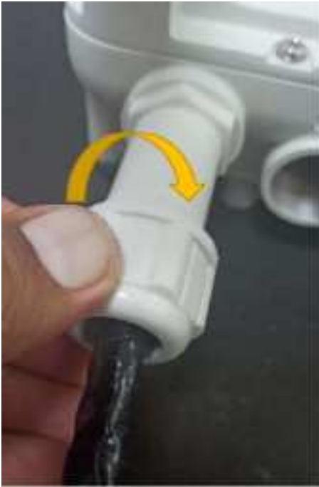
Figure 147: Fitting the gland nut
