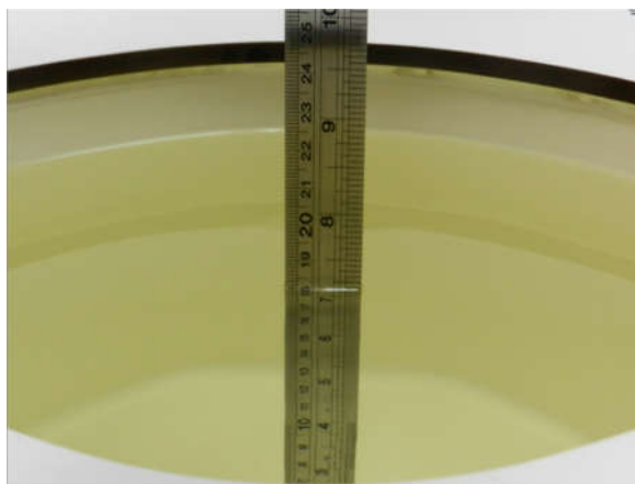
Fig 10.1 Photo of Liquid Height for Body SAR
