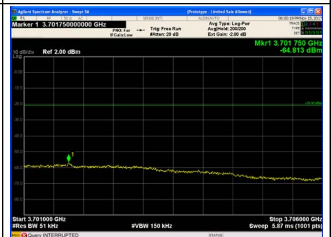
10MHz - 3701M-3706M Mid CH 64QAM
