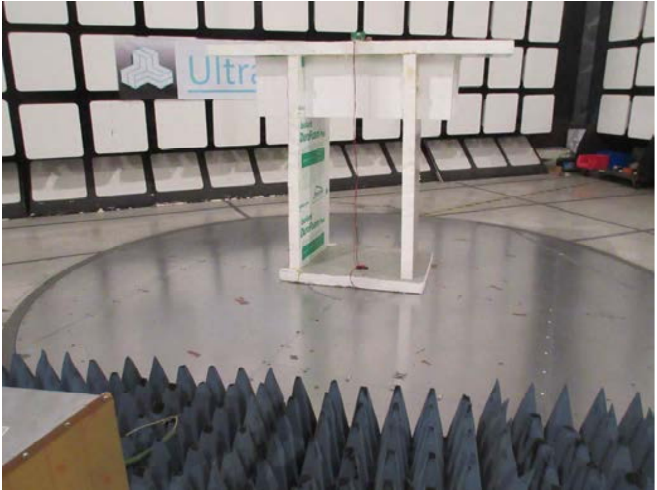
Radiated Emissions at 3 m EUT with 0 dBi \frac{1}{4} Wave Monopole Antenna, Orthogonal Position 2
