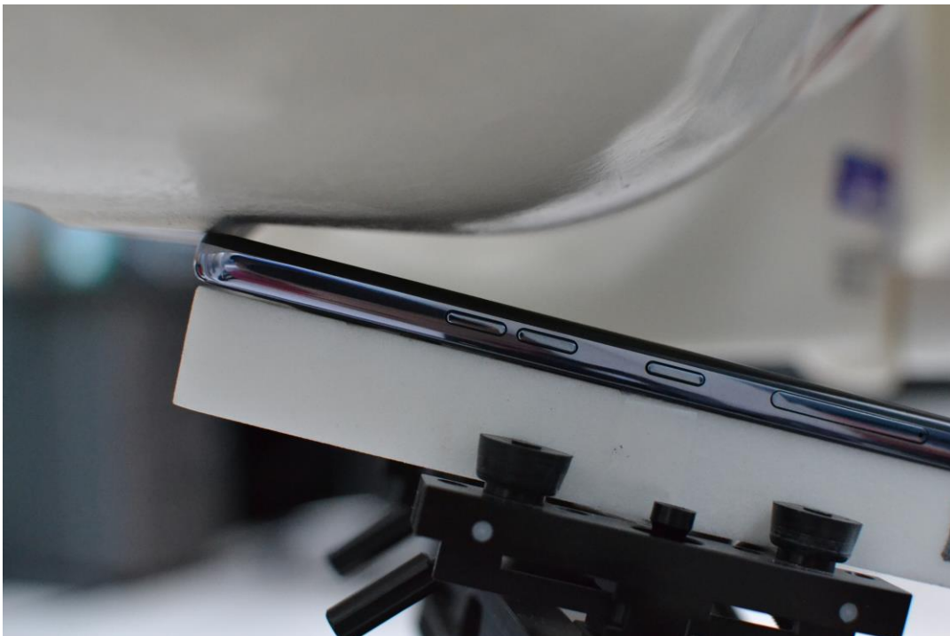
SAR Test Setup Photo 2 – Right Tilt
