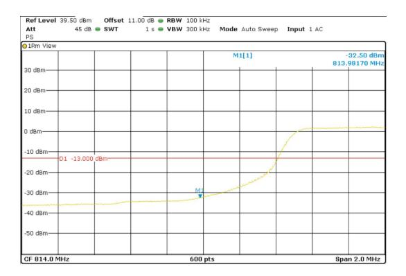
LTE QPSK MODULATION. RB = 50. Offset = 0. BW = 10 MHz
