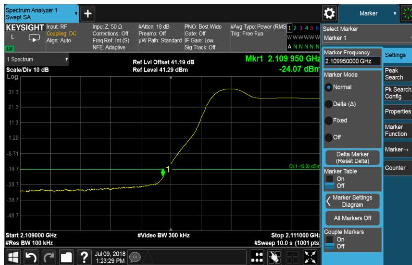
The channel power of 100kHz for 2109.975MHz is -27.49dBm, which is within the limit of -19.02dBm.
