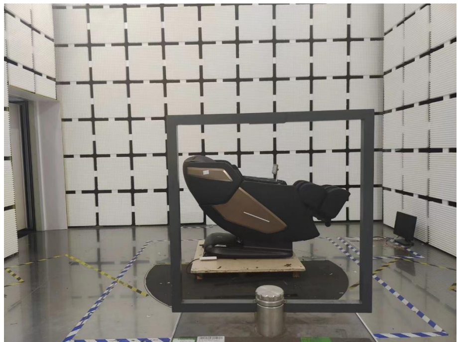
Radiation Emission Test Setup (Below 30MHz)
