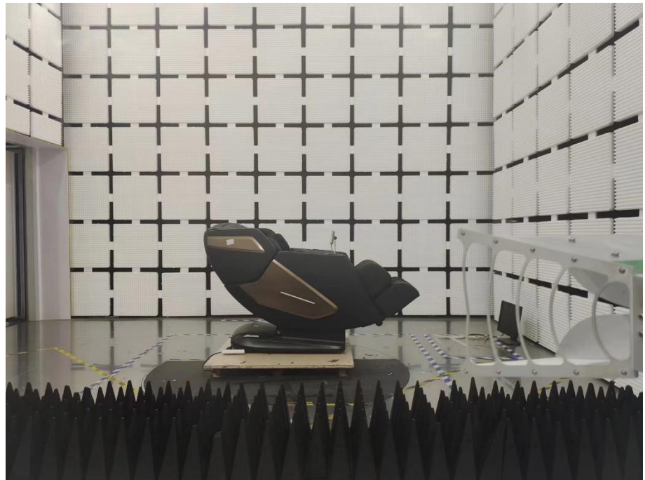
Radiation Emission Test Setup (30MHz to 1GHz)
