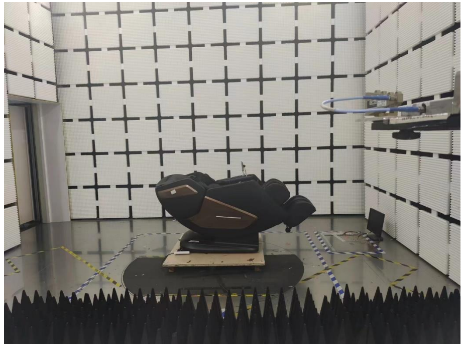
Radiation Emission Test Setup (Above 18GHz)
