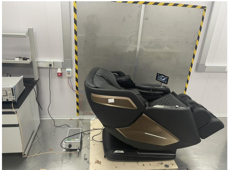
Conducted Emission Test Setup
