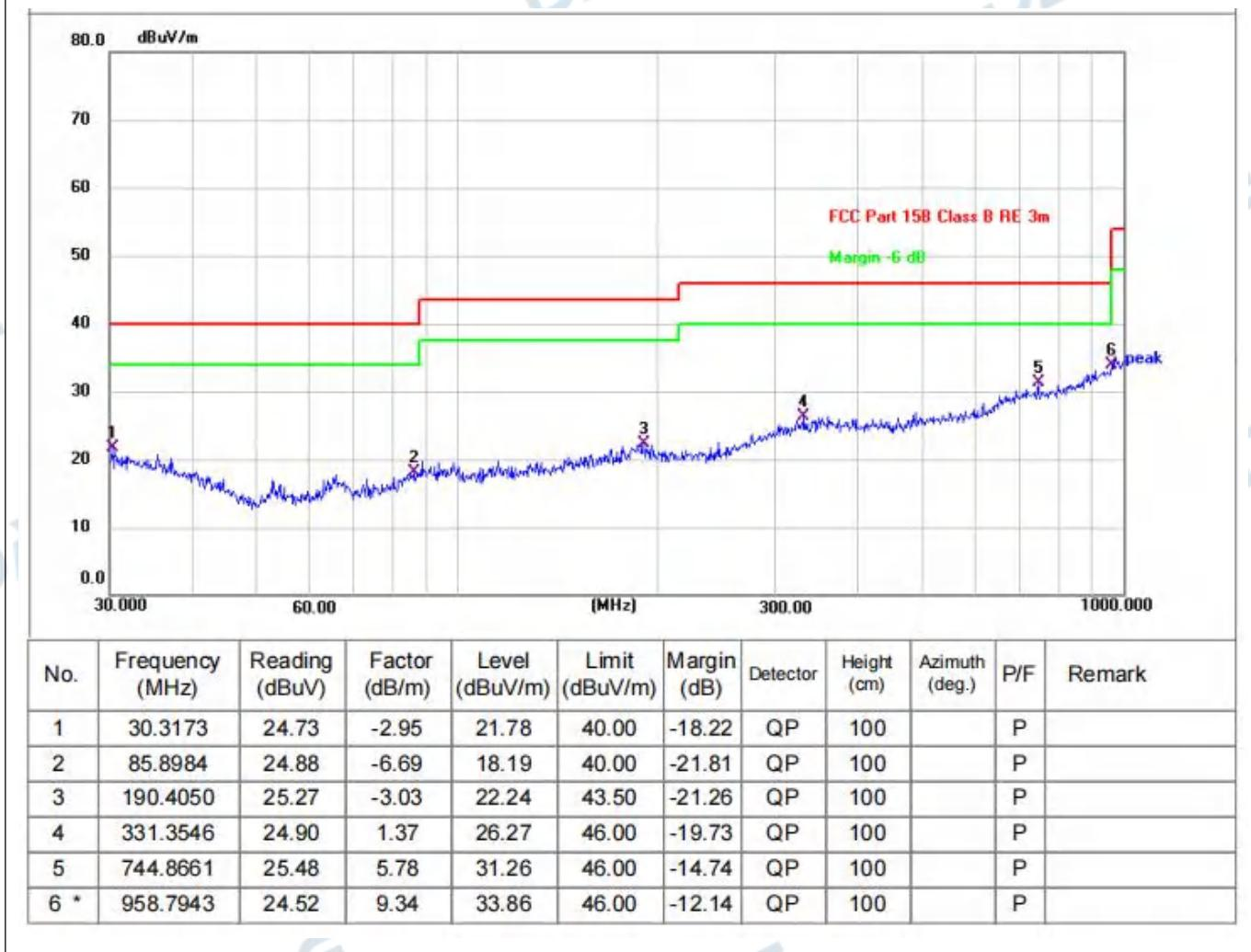
TM1 / Polarization: Vertical / Band: 2400-2483.5 MHz / BW: 20 / CH: L
