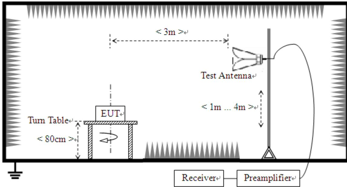
The test site semi-anechoic chamber has met the requirement of NSA tolerance 4dB according to the standards: ANSI C63.4 (2009). The EUT was set-up on insulator 80cm above the Ground Plane. The set-up and test methods were according to ANSI C63.4.
