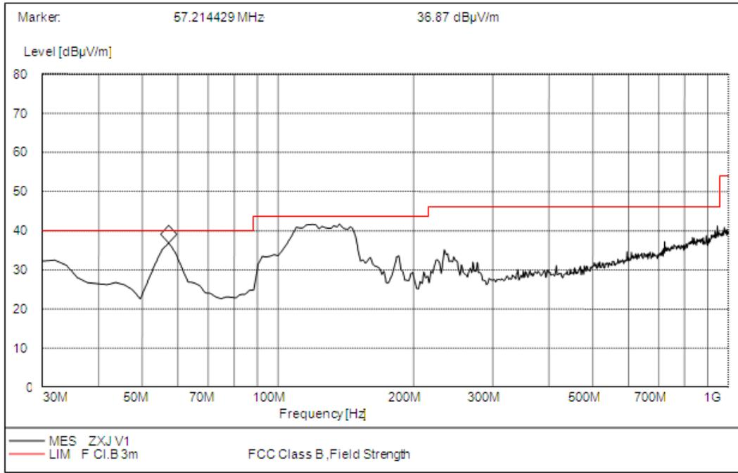
(Plot B: 30MHz to 1GHz, Antenna Vertical)
