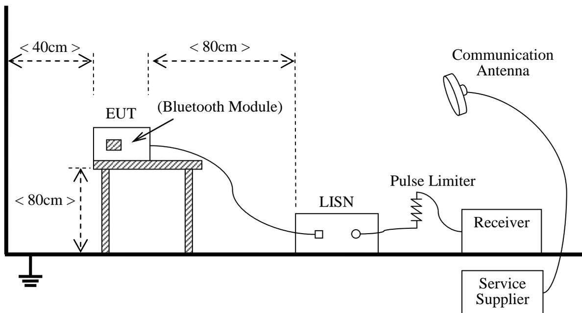
The Table-top EUT was placed upon a non-metallic table 0.8m above the horizontal metal reference ground plane. EUT was connected to LISN and LISN was connected to reference Ground Plane. EUT was 80cm from LISN. The set-up and test methods were according to ANSI C63.4:2009
