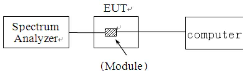
The DJI LIGHTBRIDGE of the EUT, which is powered by the Battery, is connected to the Spectrum Analyzer (SA), the path loss as the factor is calibrated to correct the reading. During the measurement, the DJI LIGHTBRIDGE of the EUT is activated.
