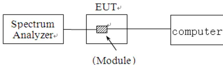
The DJI LIGHTBRIDGE of the EUT, which is powered by the Battery, is connected to the Spectrum Analyzer (SA), the path loss as the factor is calibrated to correct the reading. During the measurement, the DJI LIGHTBRIDGE of the EUT is activated and controlled .
