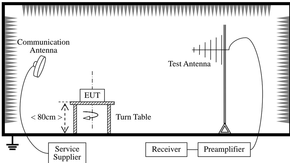
The DJI LIGHTBRIDGE of the EUT is powered by the Battery. The Module is located in a 3m Semi-Anechoic Chamber; the antenna factors, cable loss and so on of the site as factors are calculated to correct the reading. During the measurement, the DJI LIGHTBRIDGE is activated and controlled by the Bluetooth Service Supplier (SS) via a Common Antenna. For the Test Antenna:
