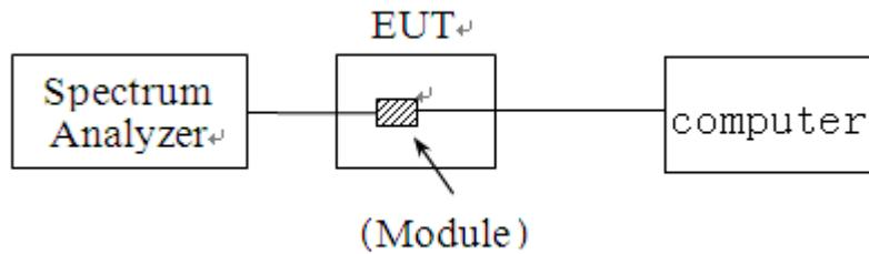
The DJI LIGHTBRIDGE of the EUT, which is powered by the Battery, is connected to the Spectrum Analyzer (SA), the path loss as the factor is calibrated to correct the reading. During the measurement, the DJI LIGHTBRIDGE of the EUT is activated.
