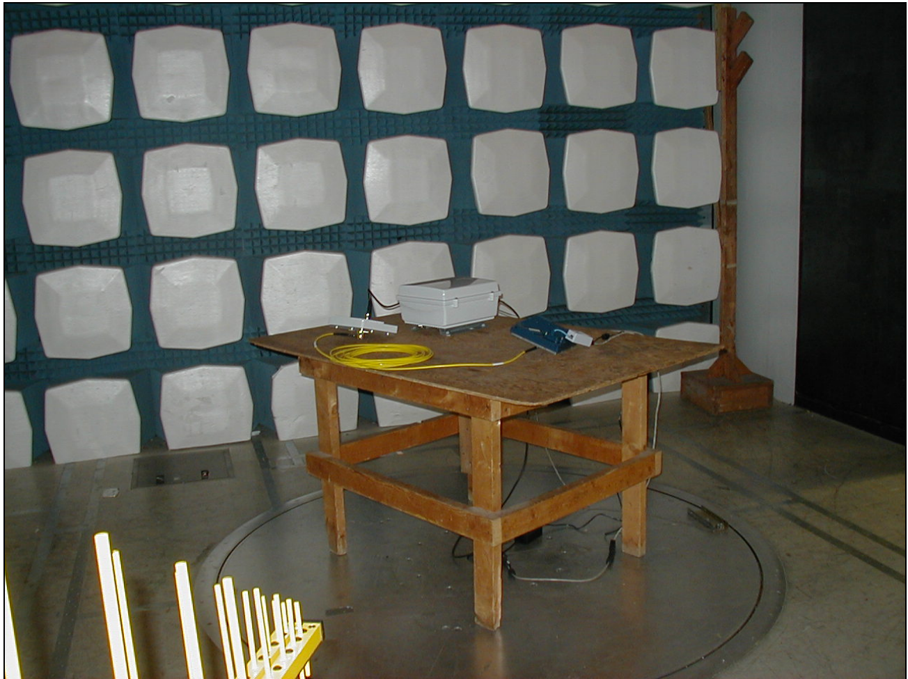
Photograph 2. Radiated Spurious Emissions, Test Set-up
