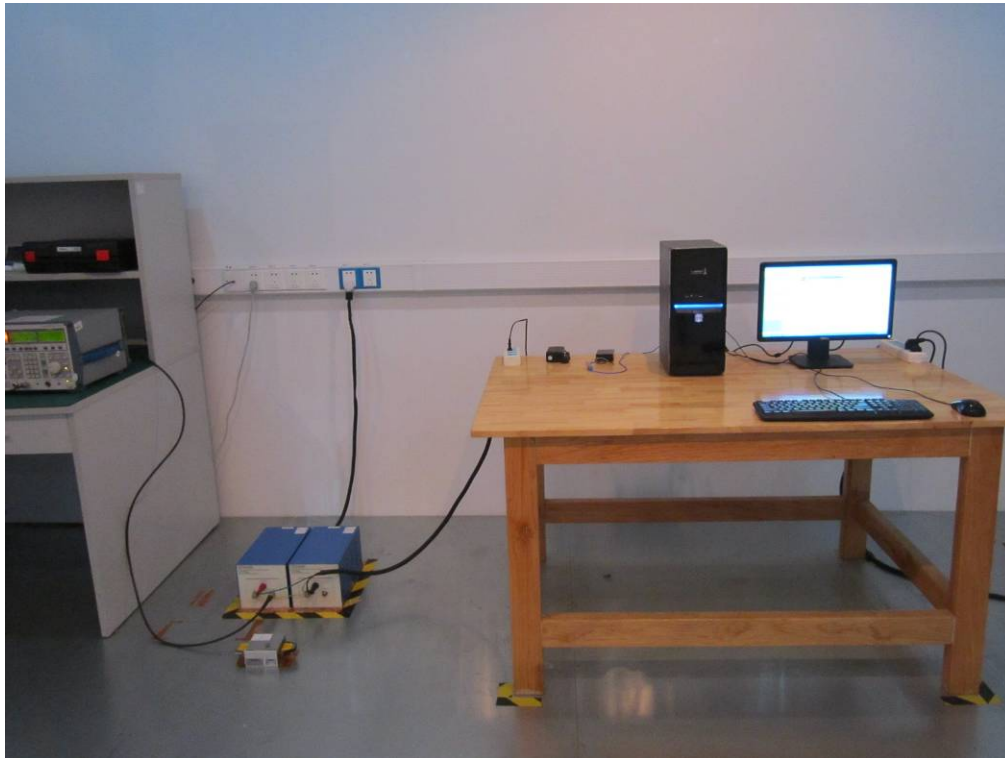
Conducted Emissions Test Setup Front View
