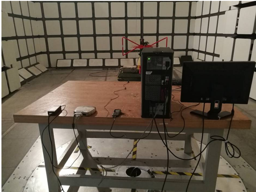
Radiated Emissions – Rear View (Below 1 GHz)
