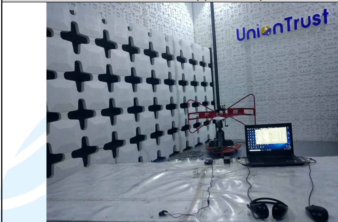
Radiated emission Test Setup (30 MHz~1 GHz) – Mode4
