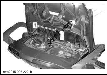
1. Label 7 is attached to tether cord, under passenger seat
