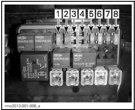
FUSES - LEFT FUSE BOX
