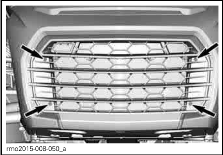
RETAINING SCREWS TO REMOVE
