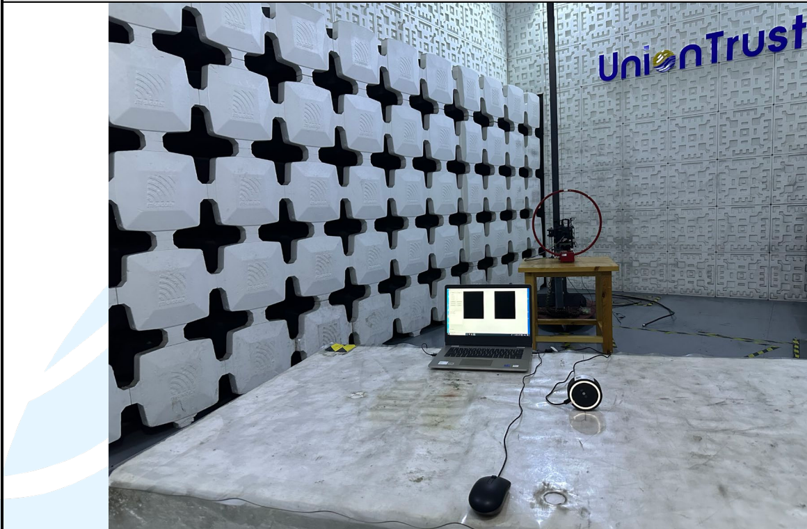
Radiated emission Test Setup (Below 30 MHz)
