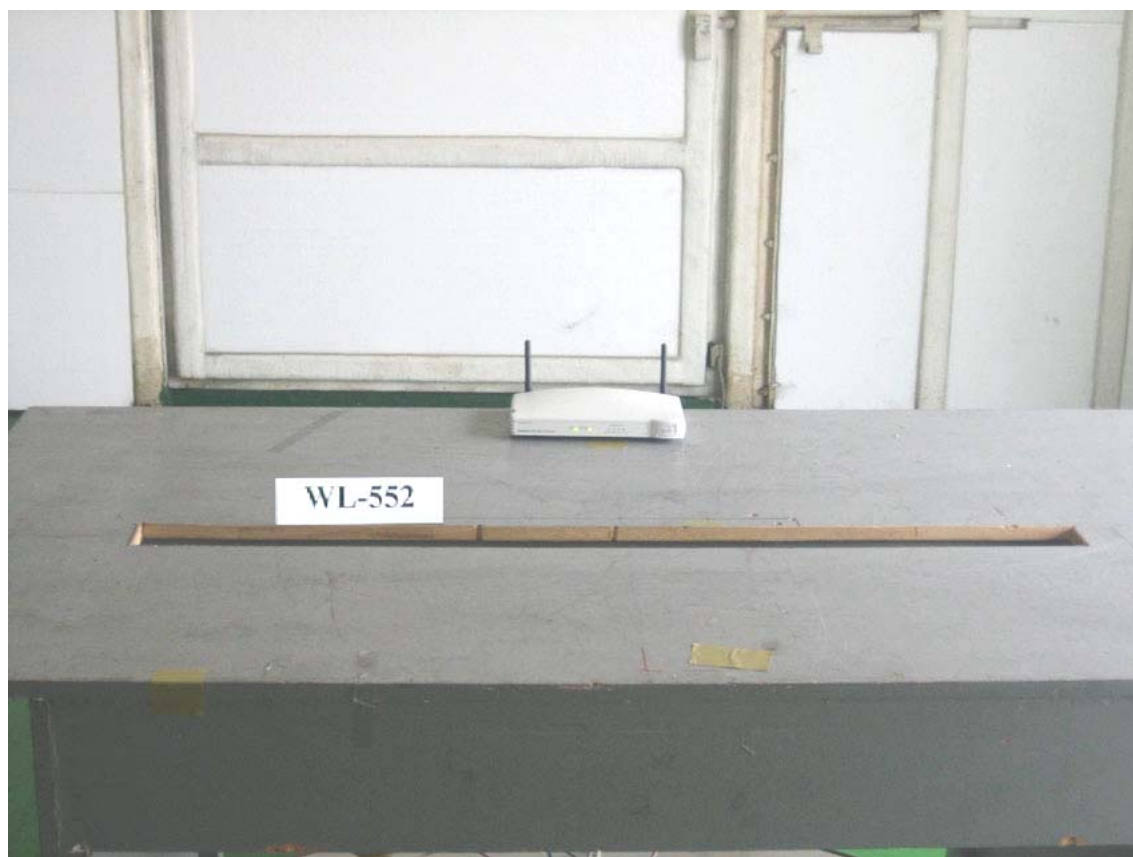
Photo 1: Radiated Emission Test Set-up
