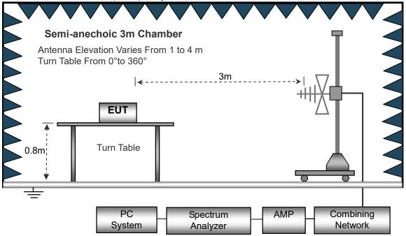
(C) Radiated Emission Test-Up Frequency Above 1GHz
