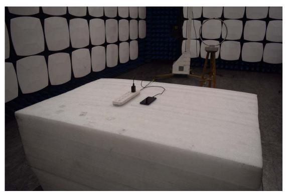
3. Radiated emission (9KHz-30MHz)
