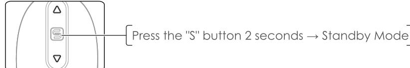
Important: Operating by the remote control (you must turn on the vibrator first): Press the S button 2 seconds to enter the standby mode (If there's no any operation within 30 minutes, the vibrator will turn off automatically). If you want to activate the vibration, just click any button on the remote control.
