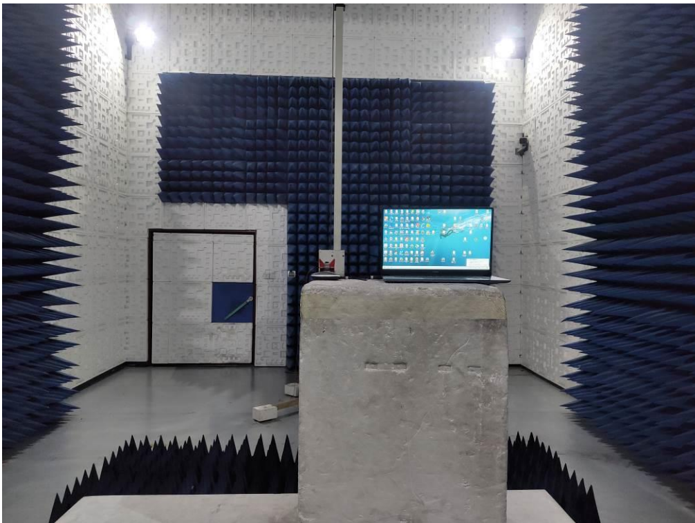
RADIATED EMISSION TEST SETUP ABOVE 1GHZ
