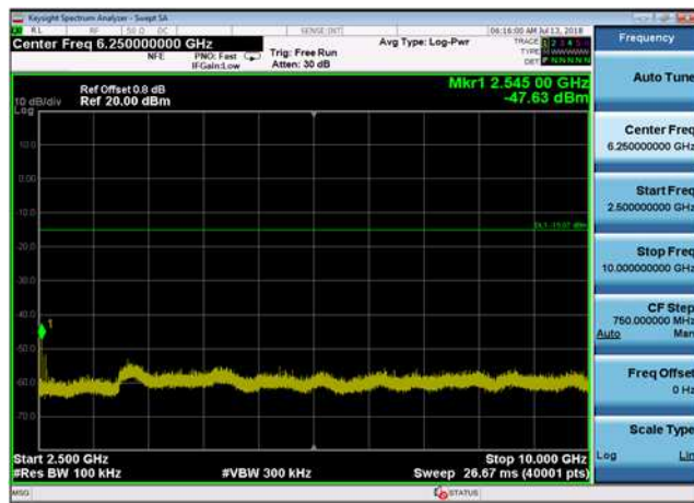
DQPSK,2480MHz,2DH5,Plot 1,Band Edge
