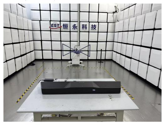
Radiated Test (Above 1GHz)
