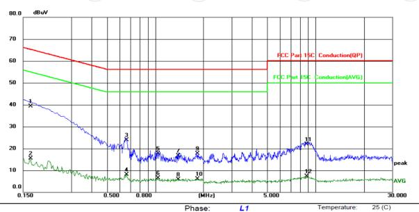
Limit: FCC Part 15C Conduction(QP) Power: Humidity: 55 %RH
