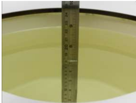
Fig 11.1 Photo of Liquid Height for Body SAR
