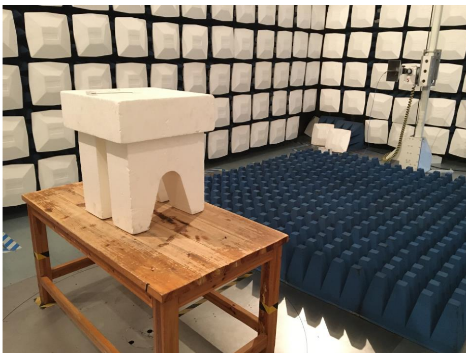
Test Setup For Radiated Emission (Above 1GHz)
