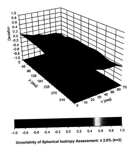
Deviation from Isotropy in Air Error (\, \, \), f = 900 MHz
