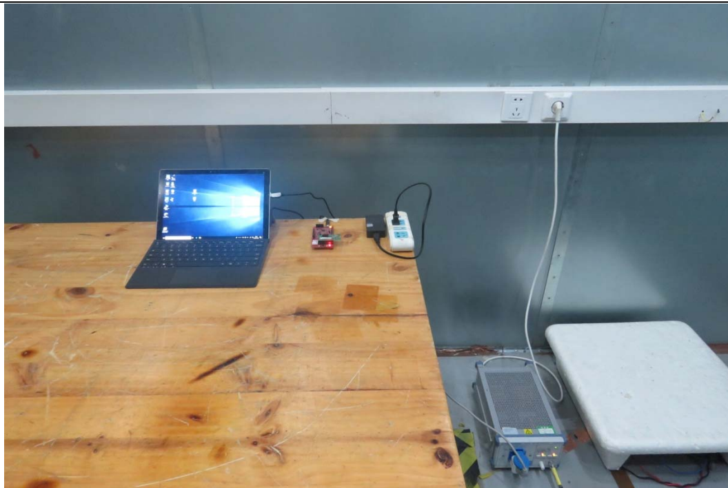
Picture 2 Conducted Emission Test Setup
