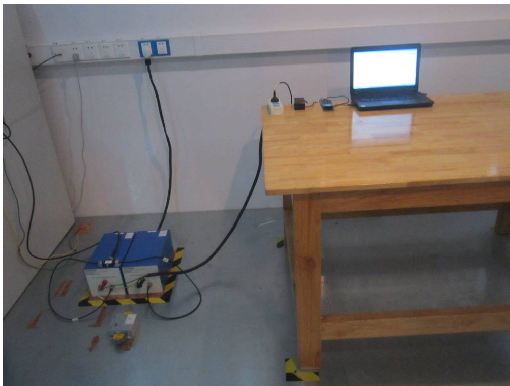
Conducted Emissions Test Setup Front View
