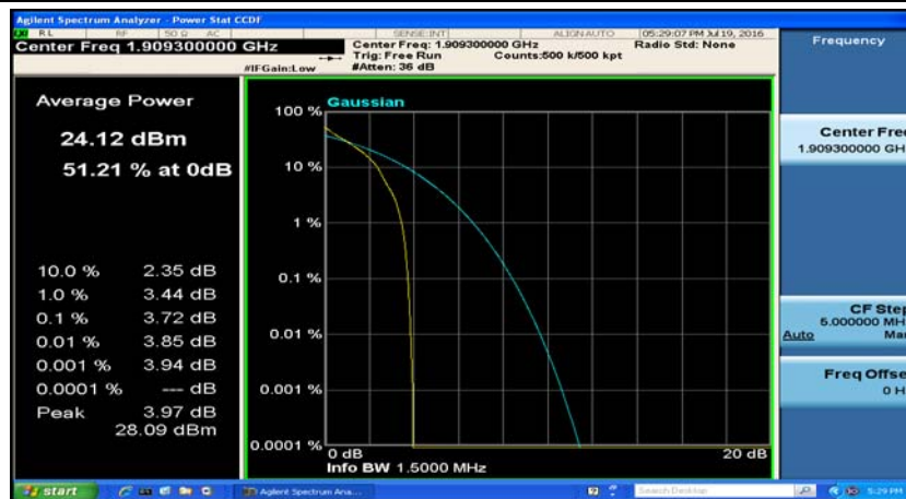
(Channel Bandwidth: 1.4 MHz)_HCH_QPSK_1RB#5
