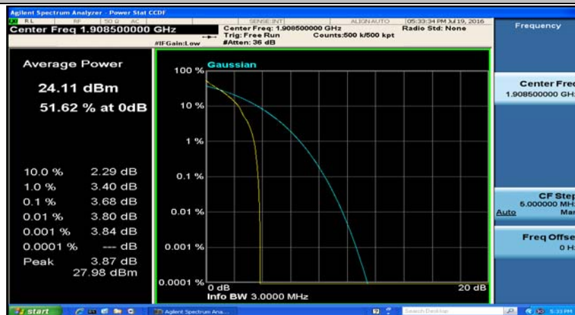
(Channel Bandwidth: 3 MHz)_HCH_QPSK_8RB#0
