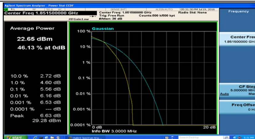
(Channel Bandwidth: 3 MHz)_LCH_16QAM_15RB#0
