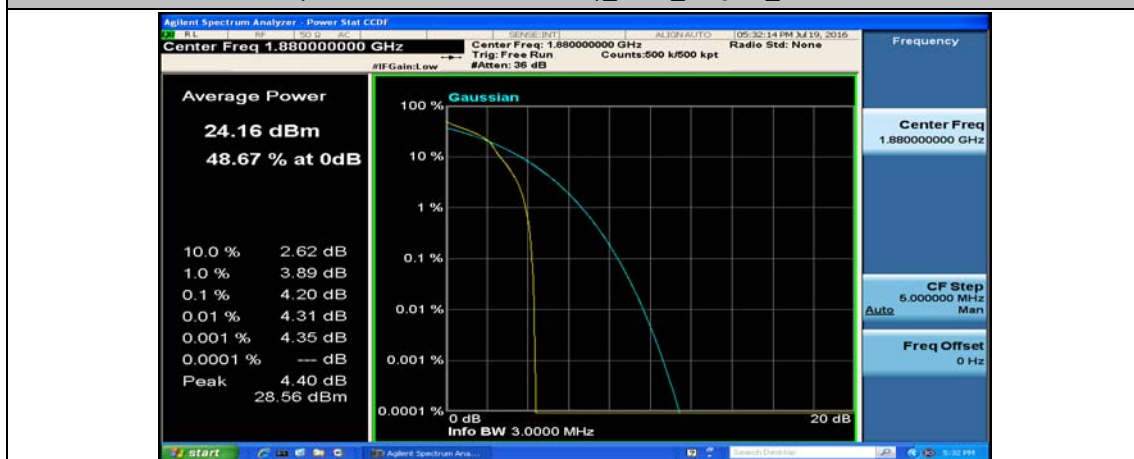
(Channel Bandwidth: 3 MHz)_MCH_16QAM_1RB#7
