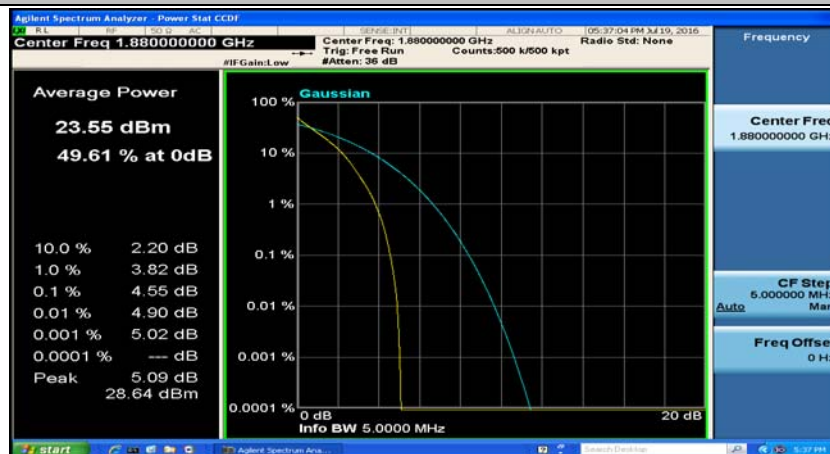
(Channel Bandwidth: 5 MHz)_MCH_QPSK_12RB#13
