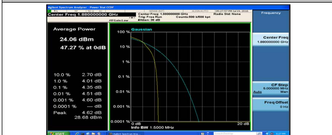
(Channel Bandwidth: 1.4 MHz)_MCH_16QAM_1RB#5
