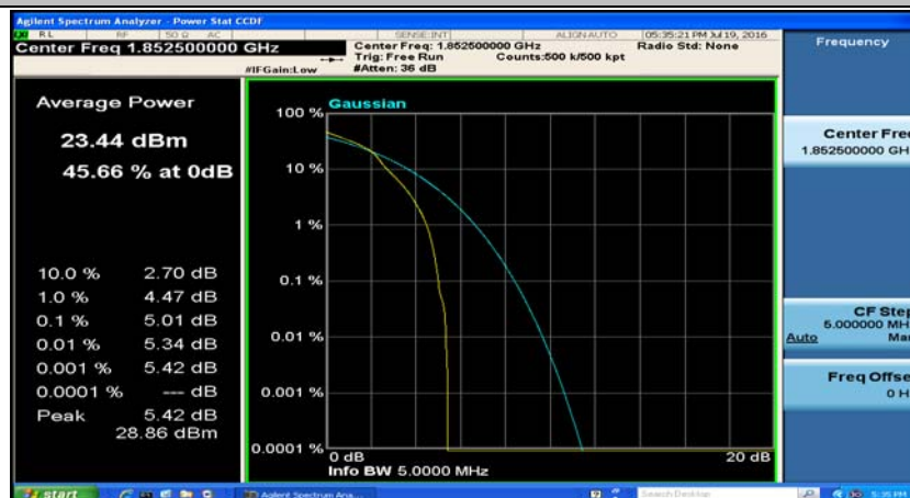
(Channel Bandwidth: 5 MHz)_LCH_16QAM_12RB#0
