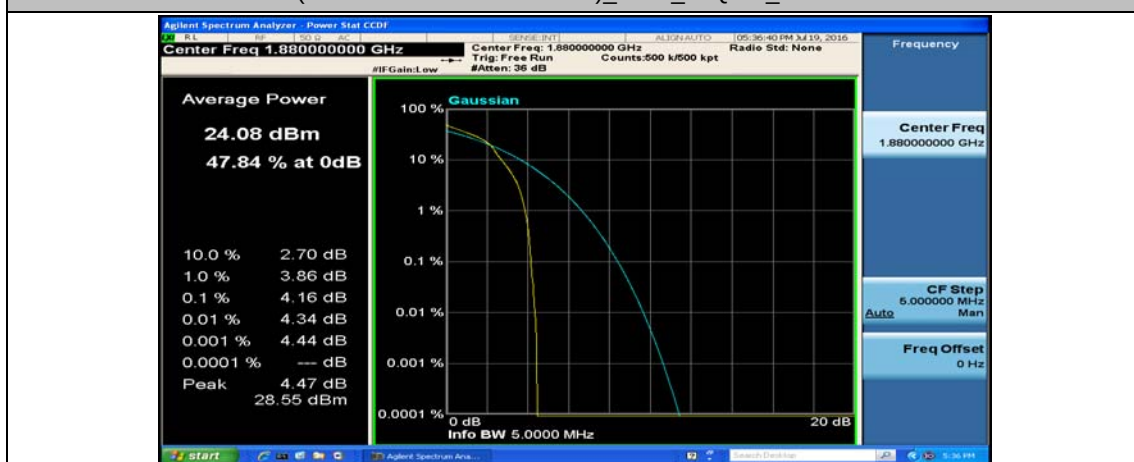
(Channel Bandwidth: 5 MHz)_MCH_16QAM_1RB#12
