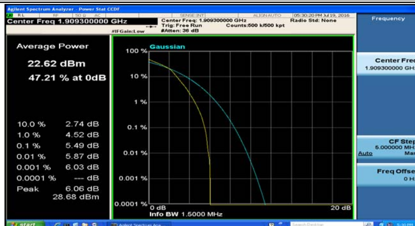
(Channel Bandwidth: 1.4 MHz)_HCH_16QAM_6RB#0
