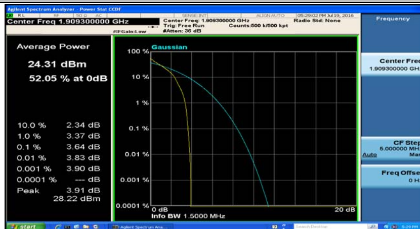
(Channel Bandwidth: 1.4 MHz)_HCH_QPSK_1RB#3
