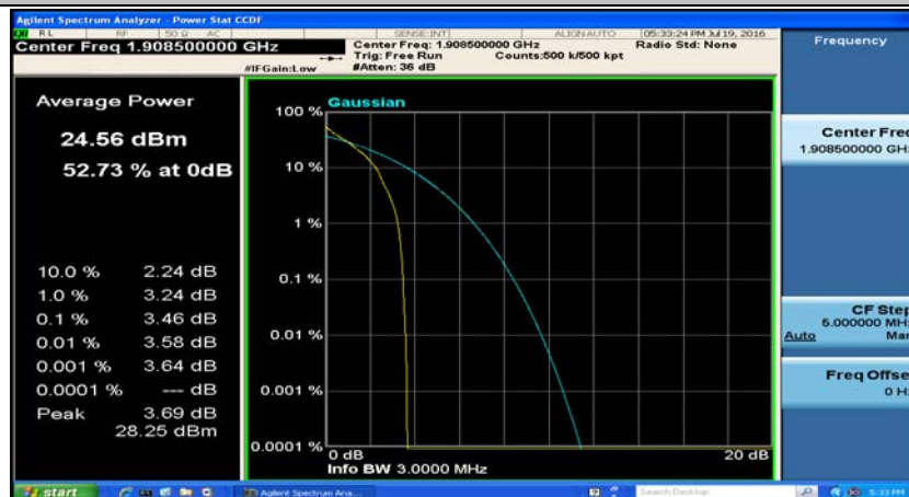
(Channel Bandwidth: 3 MHz)_HCH_QPSK_1RB#7
