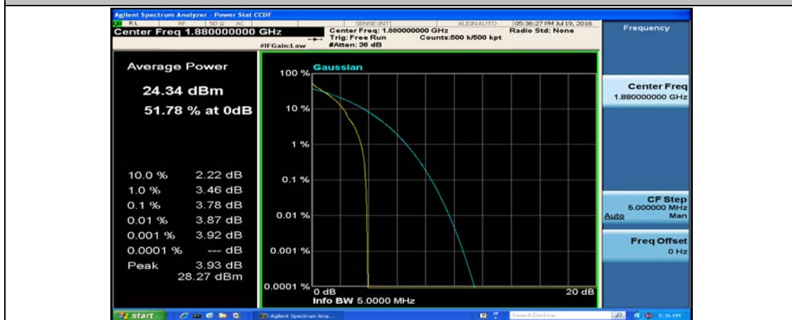
(Channel Bandwidth: 5 MHz)_MCH_QPSK_1RB#24
