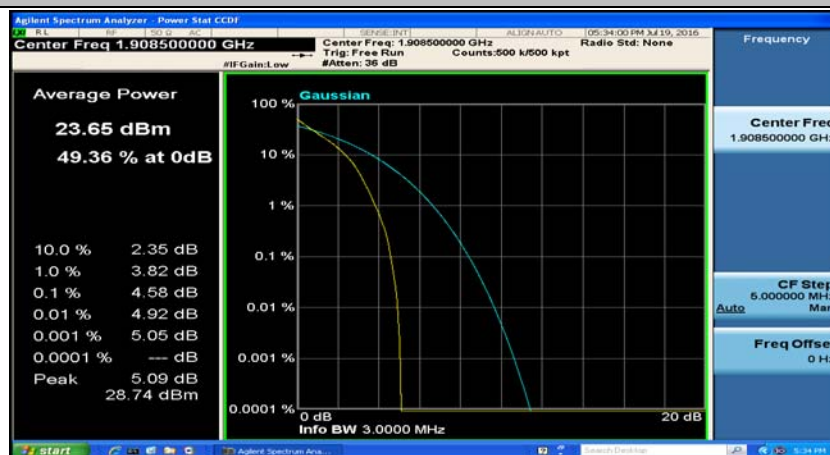
(Channel Bandwidth: 3 MHz)_HCH_QPSK_8RB#4
