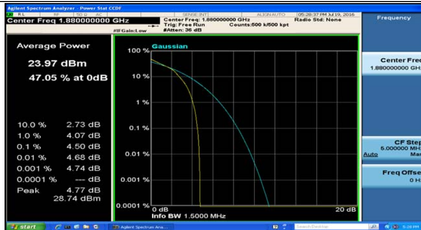
(Channel Bandwidth: 1.4 MHz)_MCH_16QAM_6RB#0
