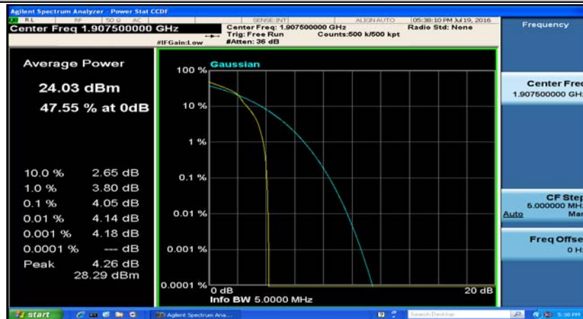
(Channel Bandwidth: 5 MHz)_HCH_16QAM_1RB#12
