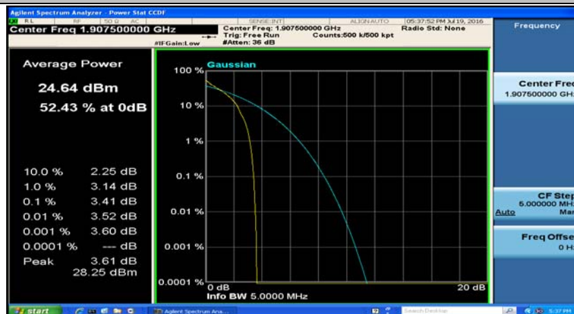
(Channel Bandwidth: 5 MHz)_HCH_QPSK_1RB#12
