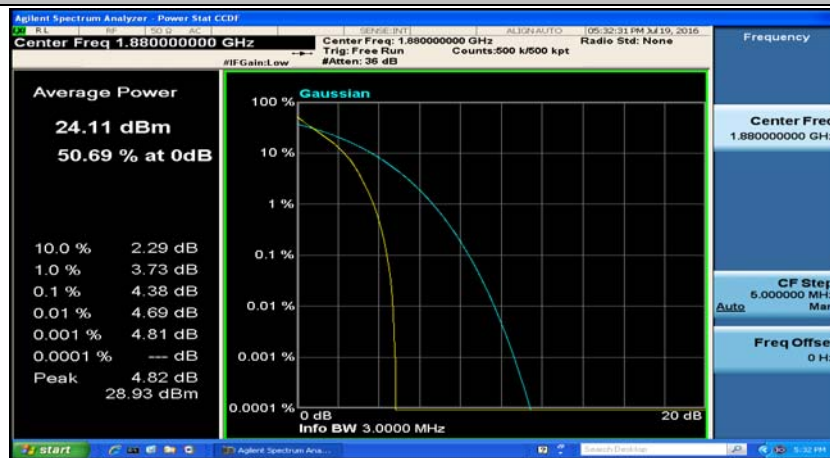
(Channel Bandwidth: 3 MHz)_MCH_QPSK_8RB#4
