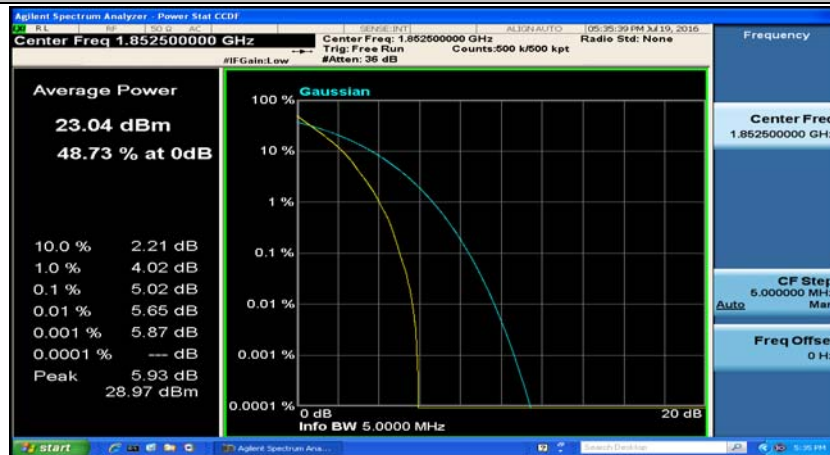
(Channel Bandwidth: 5 MHz)_LCH_QPSK_25RB#0
