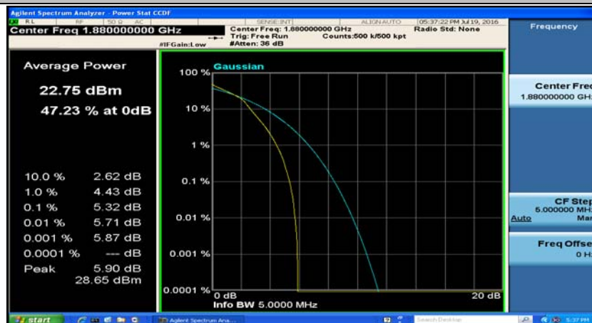
(Channel Bandwidth: 5 MHz)_MCH_16QAM_12RB#13
