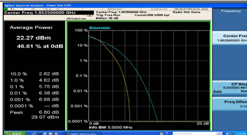
(Channel Bandwidth: 5 MHz)_LCH_16QAM_25RB#0
