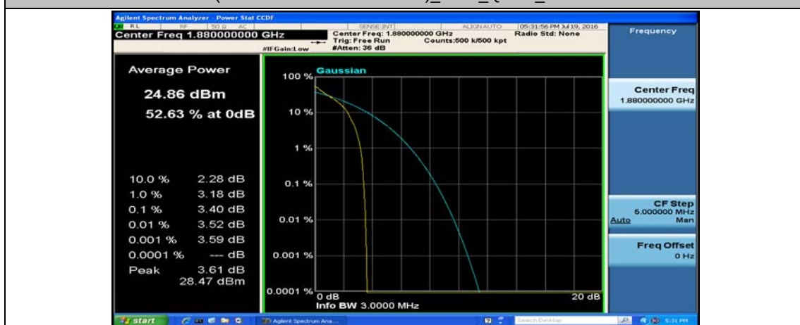
(Channel Bandwidth: 3 MHz)_MCH_QPSK_1RB#7
