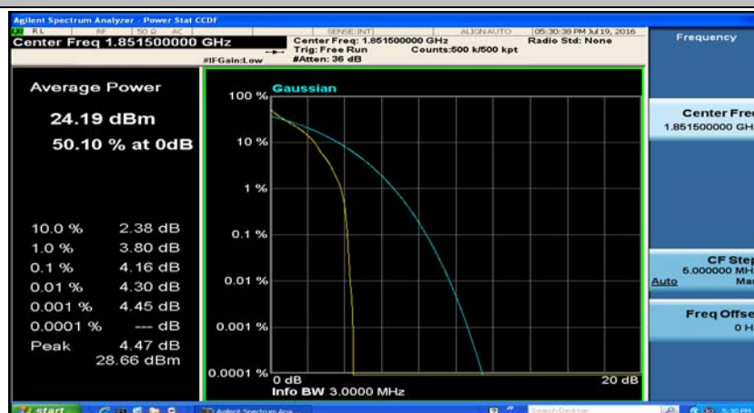
(Channel Bandwidth: 3 MHz)_LCH_QPSK_8RB#0
