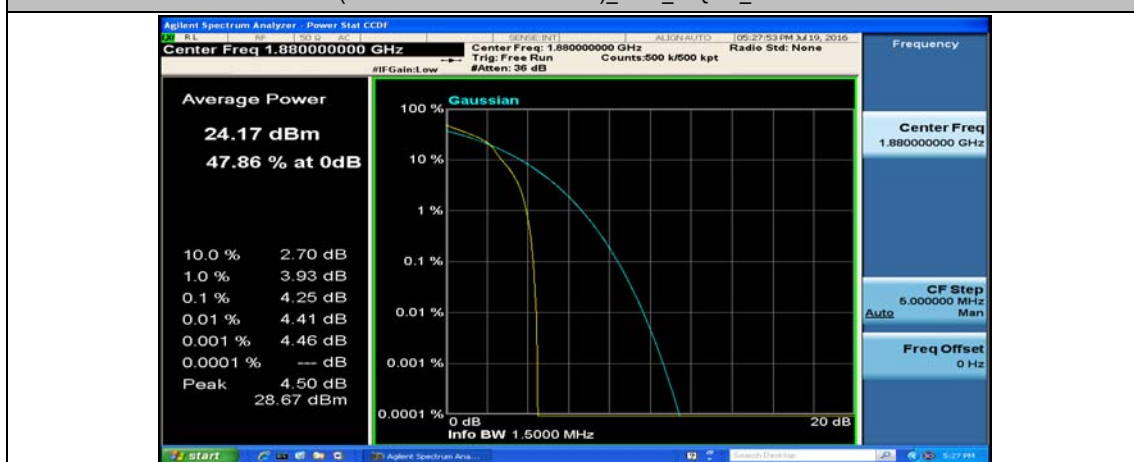
(Channel Bandwidth: 1.4 MHz)_MCH_16QAM_1RB#3
