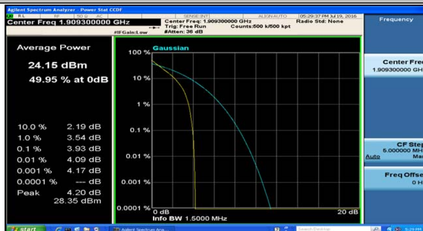
(Channel Bandwidth: 1.4 MHz)_HCH_QPSK_3RB#2
