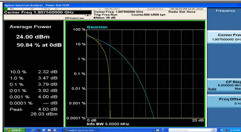
(Channel Bandwidth: 5 MHz)_HCH_QPSK_12RB#0
