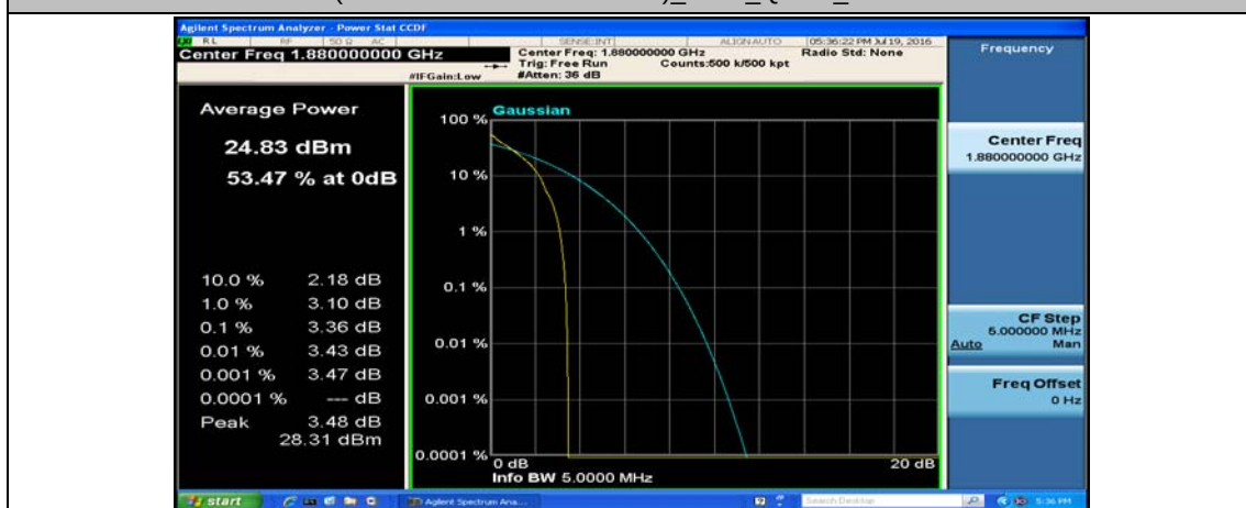
(Channel Bandwidth: 5 MHz)_MCH_QPSK_1RB#12
