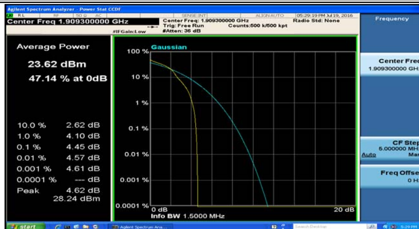
(Channel Bandwidth: 1.4 MHz)_HCH_16QAM_1RB#3
