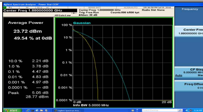
(Channel Bandwidth: 5 MHz)_MCH_QPSK_12RB#6
