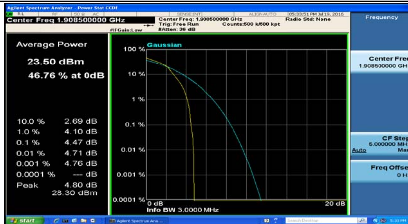
(Channel Bandwidth: 3 MHz)_HCH_16QAM_8RB#0
