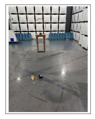
Spurious Emissions, 30 MHz to 1000 MHz; Occupied Bandwidth
