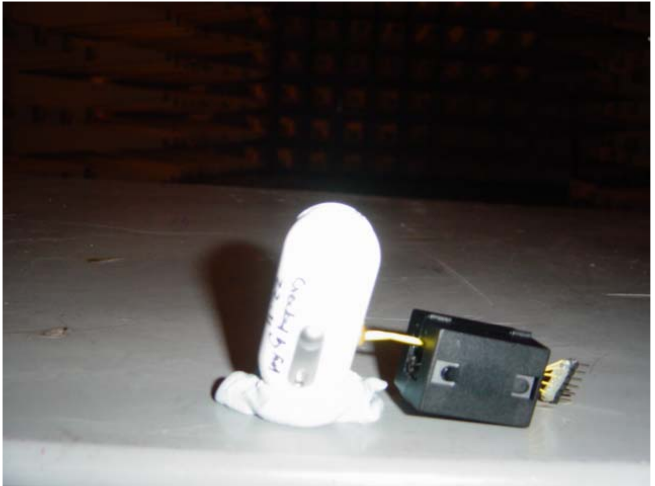
Set-up for Radiation Emission (Transceiver)
