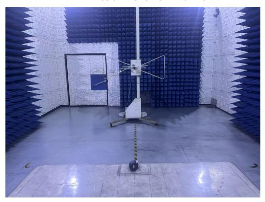
RADIATED EMISSION TEST SETUP ABOVE 1GHz
