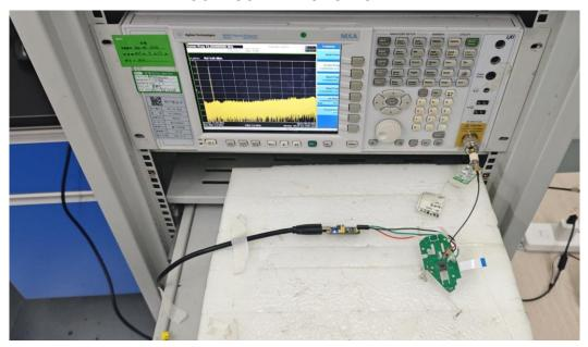
RF CONDUCTED TEST SETUP - 2.4G
