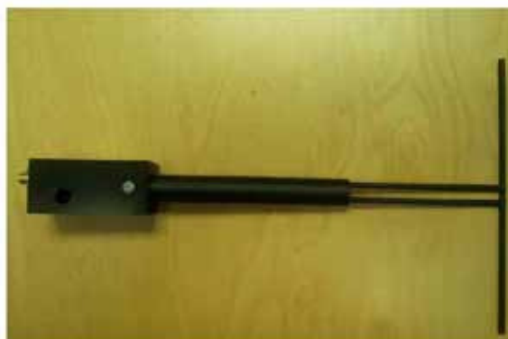
Figure 1 – MVG COMOSAR Validation Dipole
