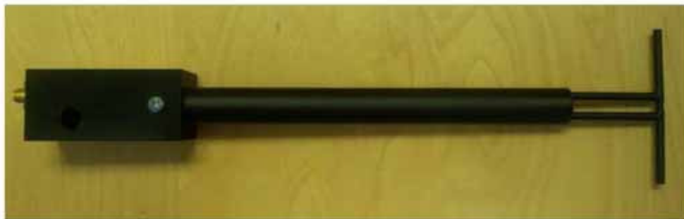
Figure 1 – MVG COMOSAR Validation Dipole
