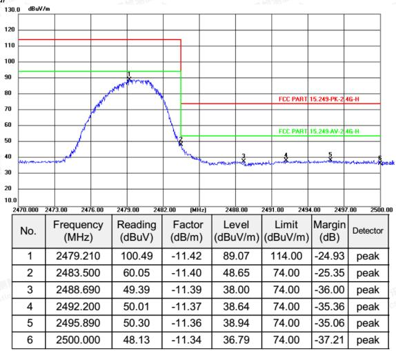
Note: Due to the measure PK emission level less than the AV limit value. No necessary to take down the AV emission level.
