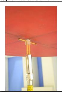
Construction: Symmetrical dipole with I/4 balun Enables
