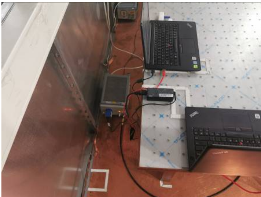
Conducted Emissions Test Setup (with charger)
