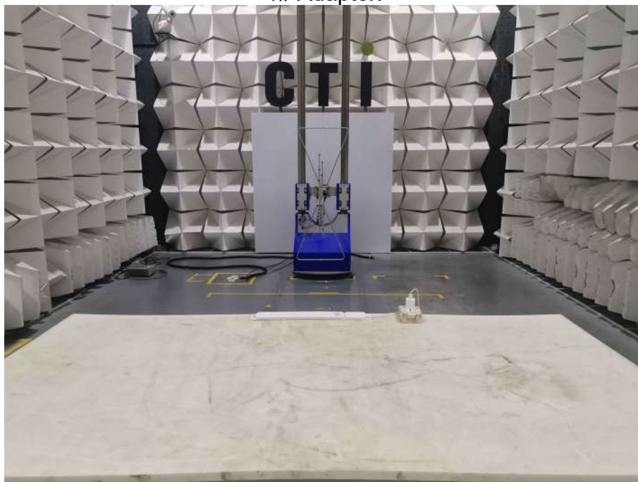
Radiated spurious emission Test Setup-1(Below 1GHz)
