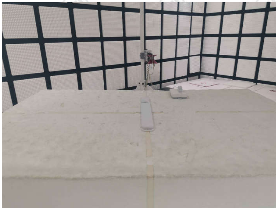
Radiated spurious emission Test Setup-2(Above 1GHz)
