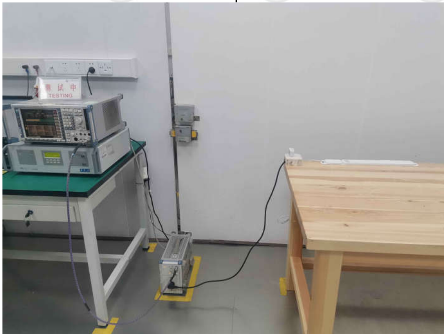
Conducted Emissions Test Setup
