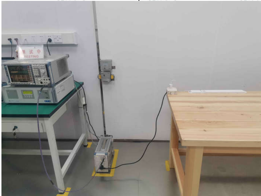
Conducted Emissions Test Setup
