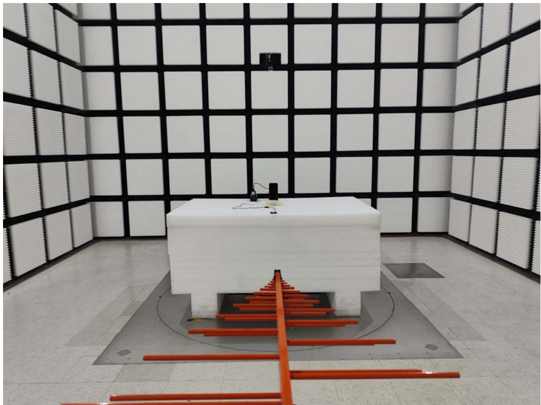
30MHz~1GHz _ Radiated Emission View-Adapter2
