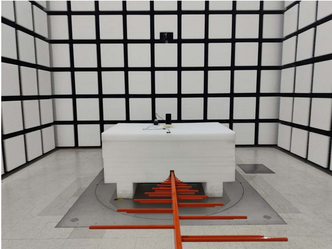
30MHz~1GHz _ Radiated Emission View-Adapter2
