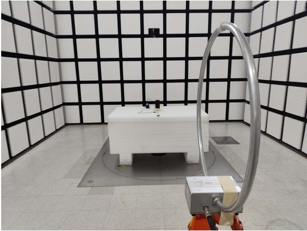
9kHz~30MHz _ Radiated Emission View - Ground-parallel Adapter2
