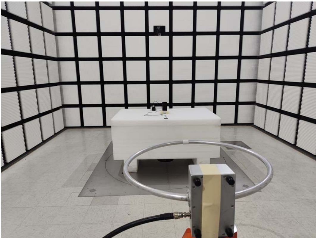
9kHz~30MHz _ Radiated Emission View - Ground-parallel Adapter2
