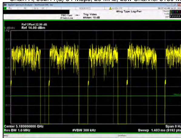
Chain A, 802.11(a) 54 Mbps, 20 MHz, Low Channel 5180 MHz
