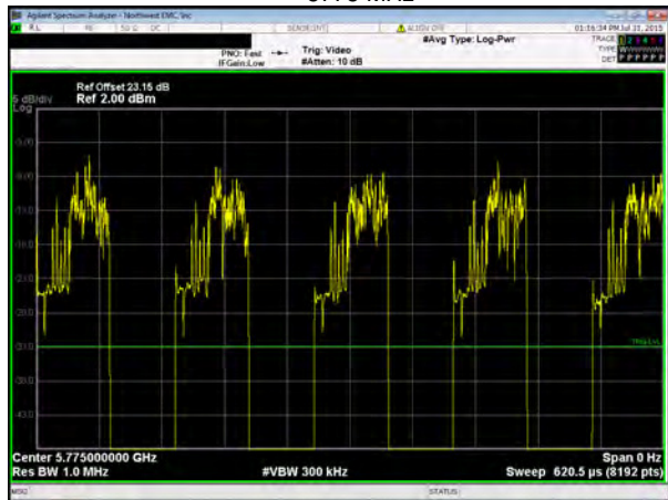
Chain A, 802.11(ac) MCS9 (256-QAM), 80 MHz, Low Channel 5775 MHz
