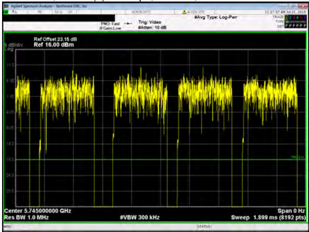
Chain A, 802.11(a) 36 Mbps, 20 MHz, Low Channel 5745 MHz
