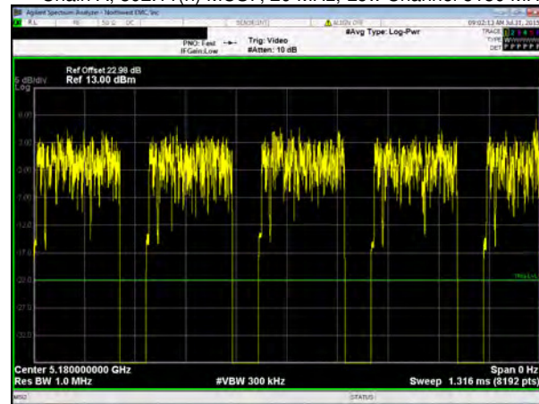
Chain A, 802.11(n) MCS7, 20 MHz, Low Channel 5180 MHz
