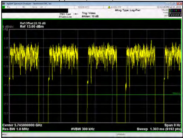
Chain A, 802.11(n) MCS7, 20 MHz, Low Channel 5745 MHz
