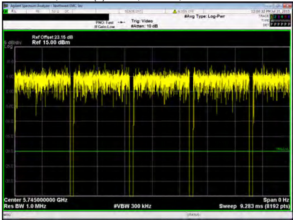
Chain A, 802.11(n) MCS0, 20 MHz, Low Channel 5745 MHz
