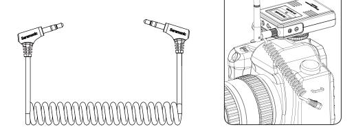
When connecting to a smartphone, tablet or computer, please use the 3.5mm TRS to TRRS (CTIA standard) output cable. Plug the 90 degree right angle TRS into the line output jack of the receiver and plug the straight TRRS end into the 3.5mm headphone jack of a smartphone, tablet, or computer.
