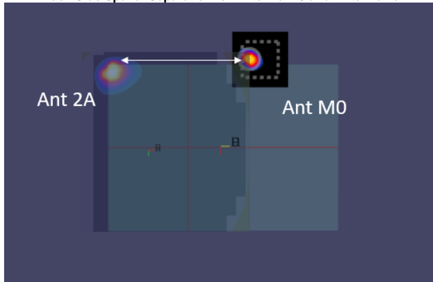
Figure C-3 Back Side Spatial Separation for Antenna M0 and Antenna 2a
