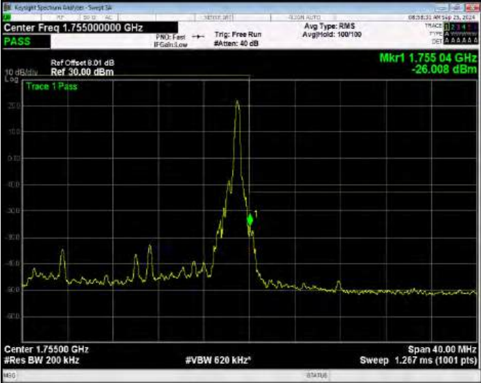
Band4 QPSK BW=20MHz Channel=20300 RB Size=100 Position=#0 Normal
