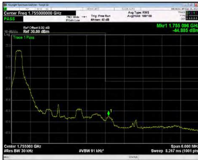
Band4 QPSK BW=3MHz Channel=20385 RB Size=1 Position=#Max Normal
