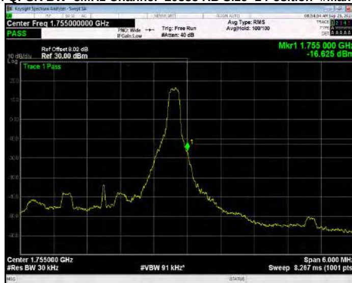
Band4 QPSK BW=3MHz Channel=20385 RB Size=15 Position=#0 Normal
