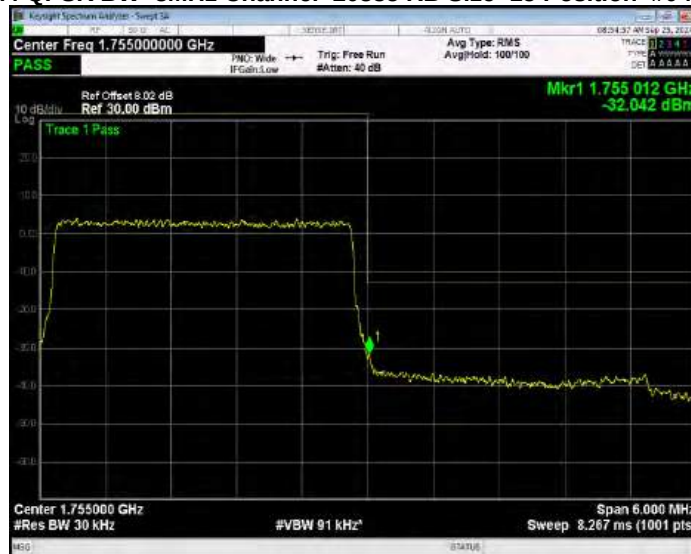
Band4 QPSK BW=3MHz Channel=20385 RB Size=15 Position=#0 Normal
