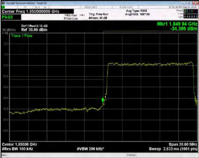
Band2 QPSK BW=10MHz Channel=18650 RB Size=50 Position=#0 Normal
