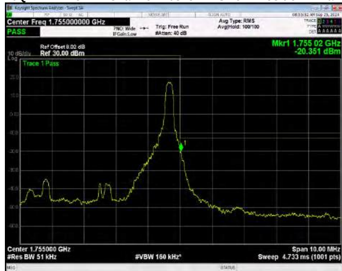
Band4 16QAM BW=5MHz Channel=20375 RB Size=25 Position=#0 Normal
