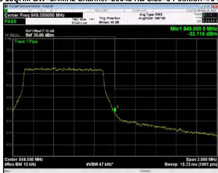
Band5 16QAM BW=1.4MHz Channel=20643 RB Size=6 Position=#0 Normal
