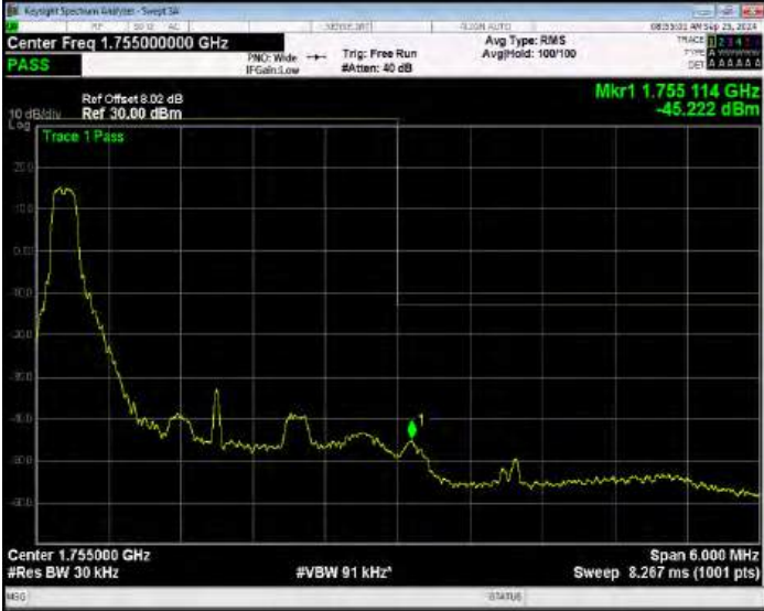
Band4 16QAM BW=3MHz Channel=20385 RB Size=1 Position=#Max Normal
