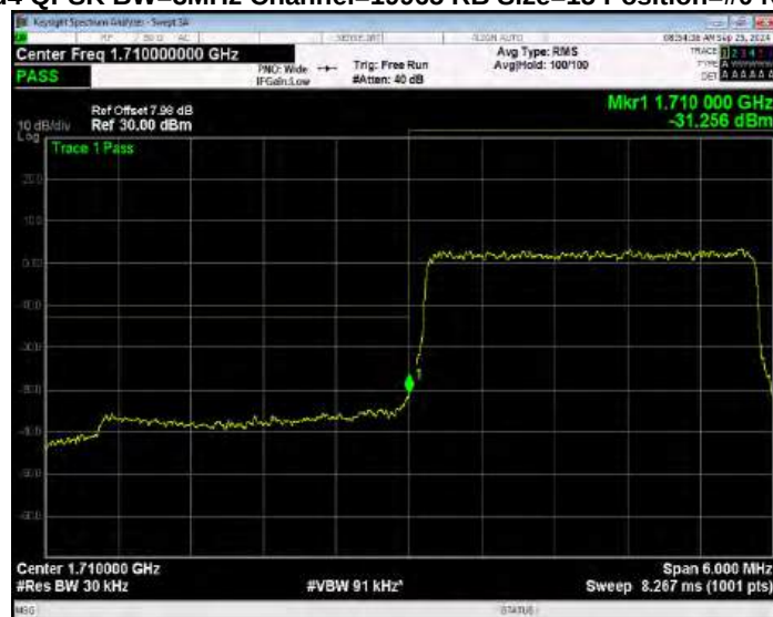
Band4 QPSK BW=3MHz Channel=19965 RB Size=15 Position=#0 Normal
