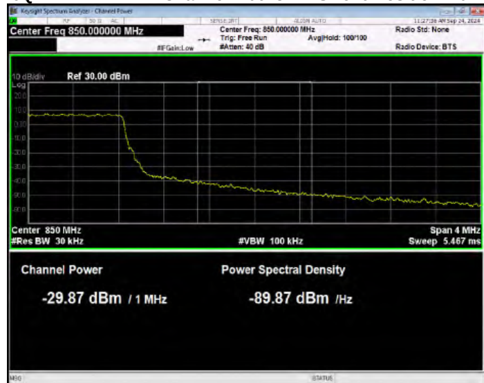
Band5 16QAM BW=1.4MHz Channel=20643 RB Size=6 Position=#0 Normal
