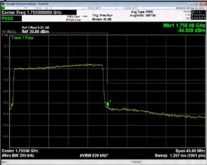
Band4 QPSK BW=20MHz Channel=20300 RB Size=100 Position=#0 Normal
