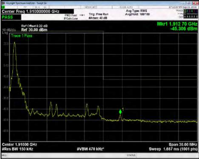
Band2 QPSK BW=15MHz Channel=19125 RB Size=1 Position=#Max Extended
