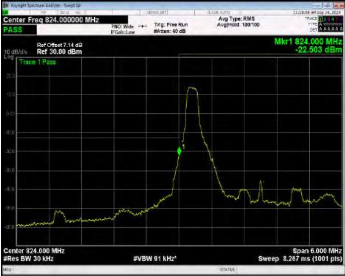
Band5 16QAM BW=3MHz Channel=20415 RB Size=1 Position=#Max Extended
