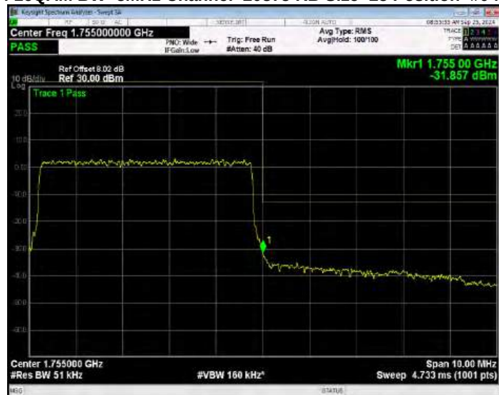
Band4 16QAM BW=5MHz Channel=20375 RB Size=25 Position=#0 Normal
