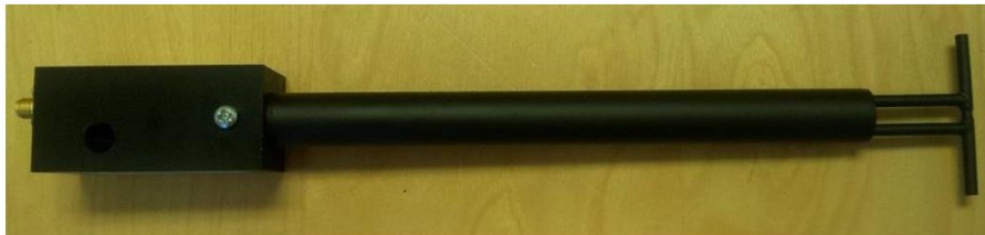
Figure 1 – MVG COMOSAR Validation Dipole
