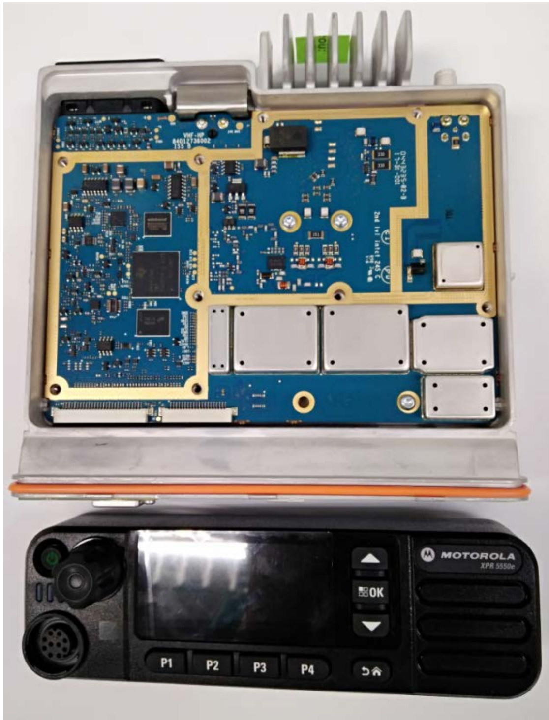
RF boards with chassis and control head (Top) (XPR5550e)
