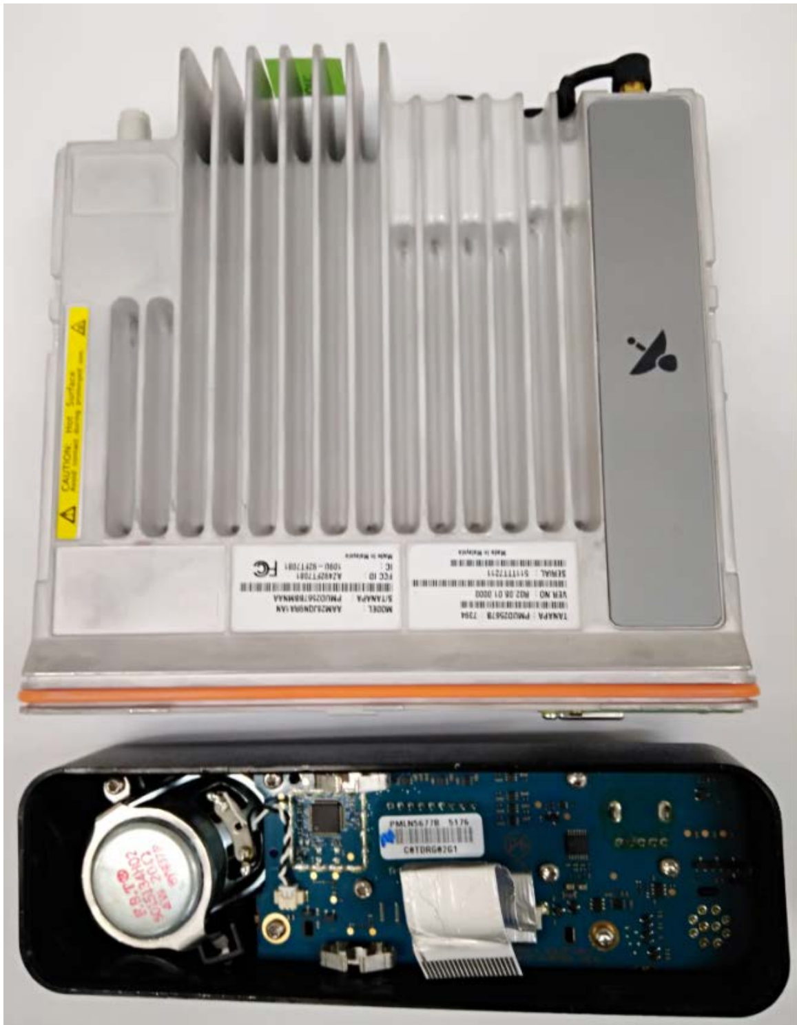
Chassis and control head (Bottom) (XPR5350e)
