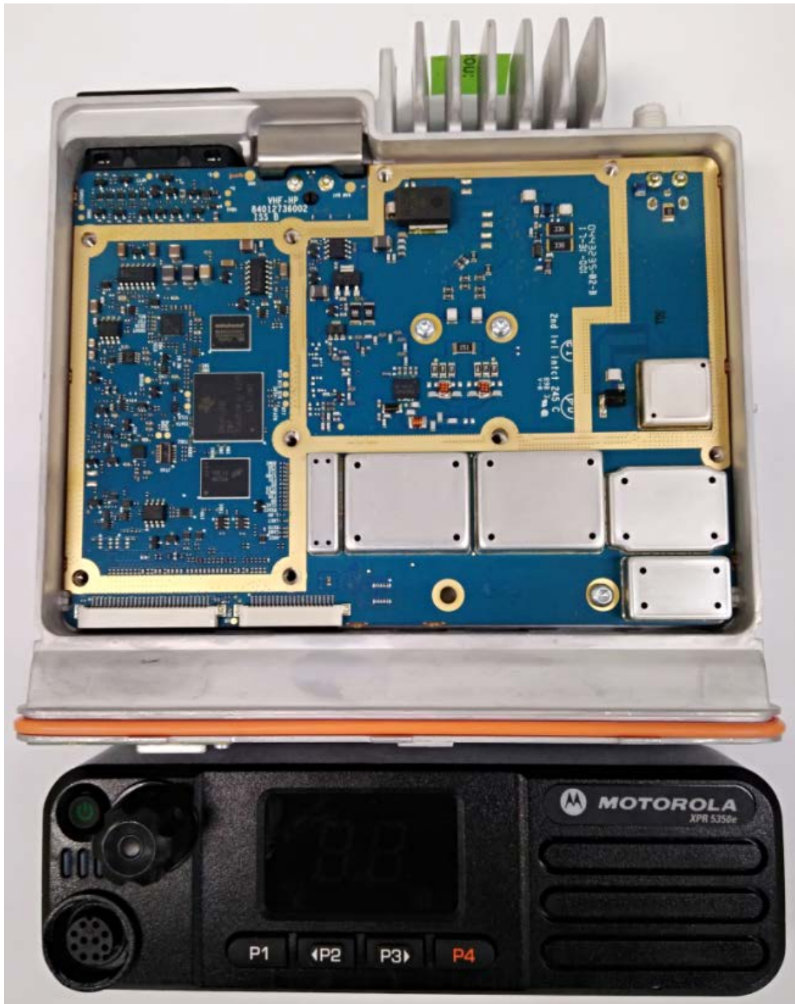
RF boards with chassis and control head (Top) (XPR5350e)
