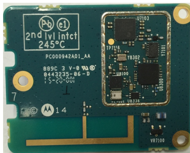
Wifi/GPS/BT board without Shield (Bottom)
