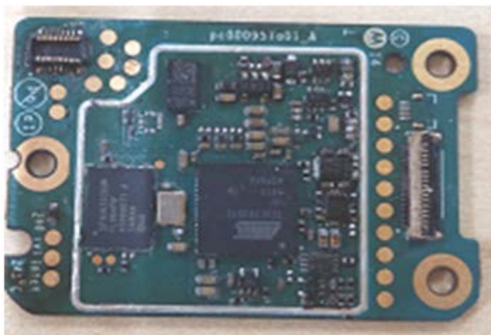
GOB board without Shield (Bottom)
