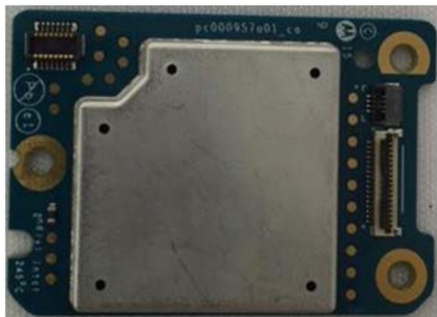
GOB board with Shield (Bottom)
