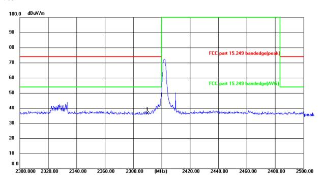
Site: 3m Anechoic Chamber Polarization: Vertical Temperature: 24.8(°C) Humidity: 51 %
