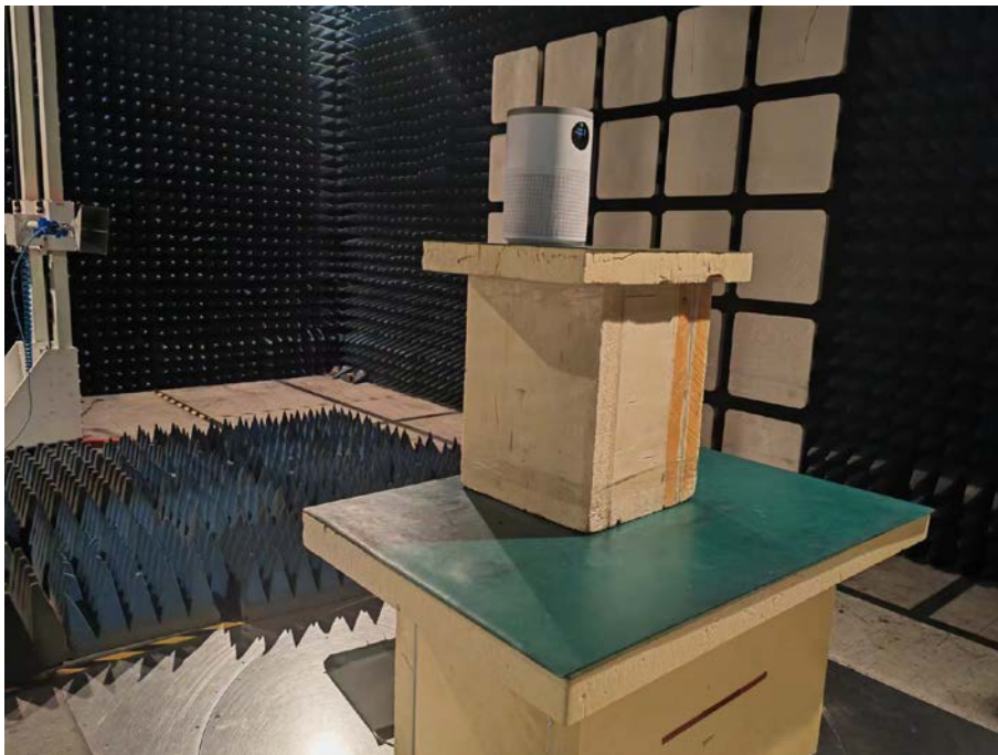
Spurious Emission Test Setup (Above 1GHz)
