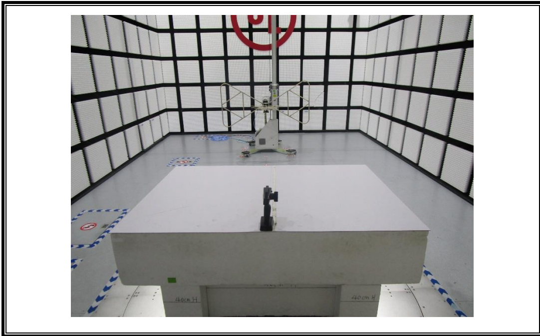
RADIATED RF MEASUREMENT SETUP (30MHz ~ 1 GHz)
