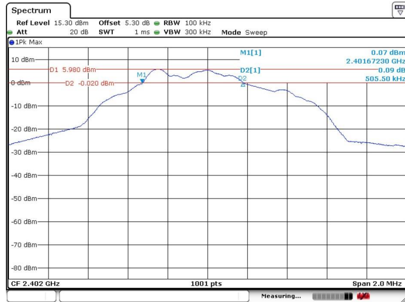
6 dB Bandwidth Plot on Channel 00
