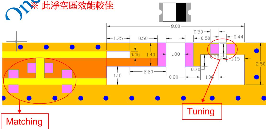
◆ 3<sup>rd</sup> Layout Dimensions in Clearance area (Size=6.0\*2.5mm)
